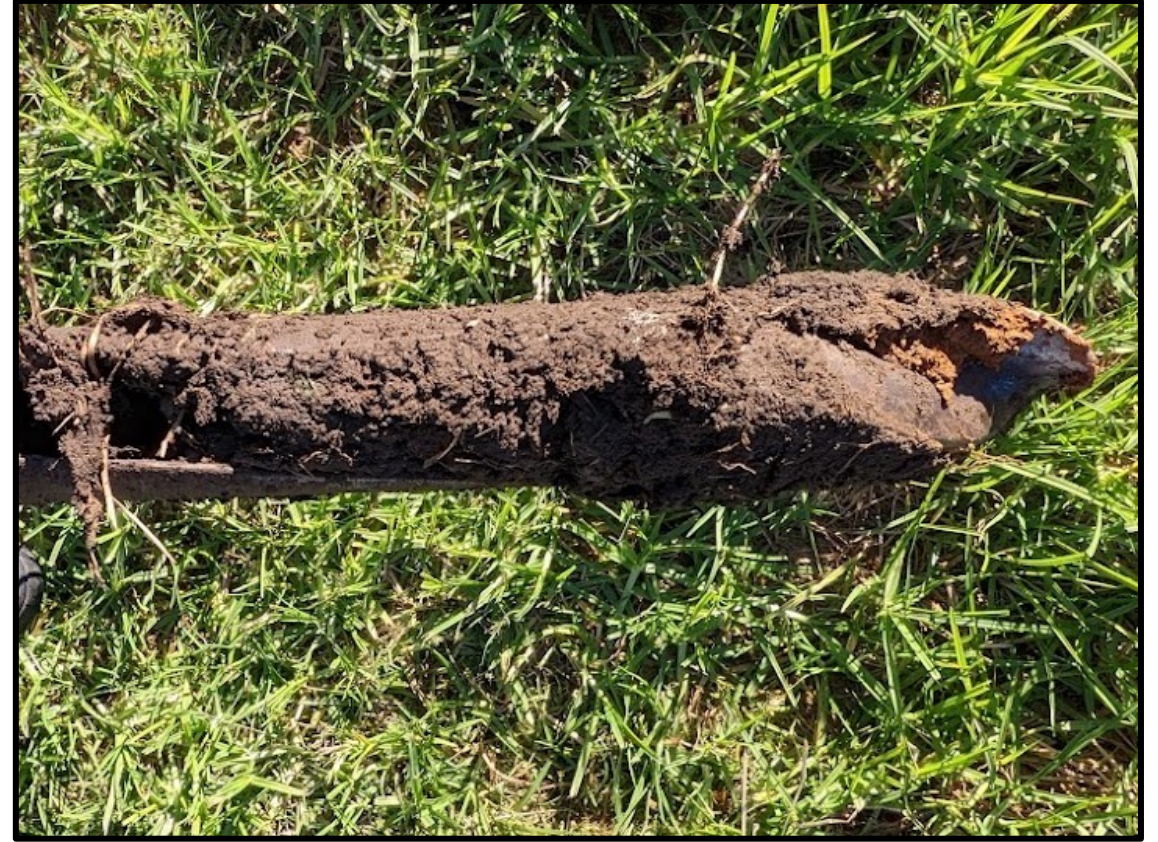
Figure 23. BH5 sample profile consisted of brown medium clay and moist soil.
